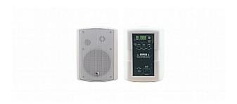
The Tavor 5-O is a pair of 5.25-inch powered two-way speakers designed for indoor wall mounting. The active speaker accepts a line-level stereo input and amplifies it using a built-in amplifier and outputs a speaker signal to the passive speaker.
